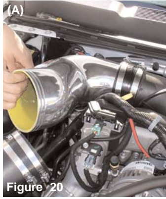
Figure 19 The cast intake is lowered and aligned with the step hose over the turbo inlet.
