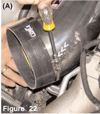
Figure 20 Once you have aligned the cast intake to the step hose, continue to press the intake into the hose (A) The power-band on the intake side is semi-tightened to hold the intake in place (B).
