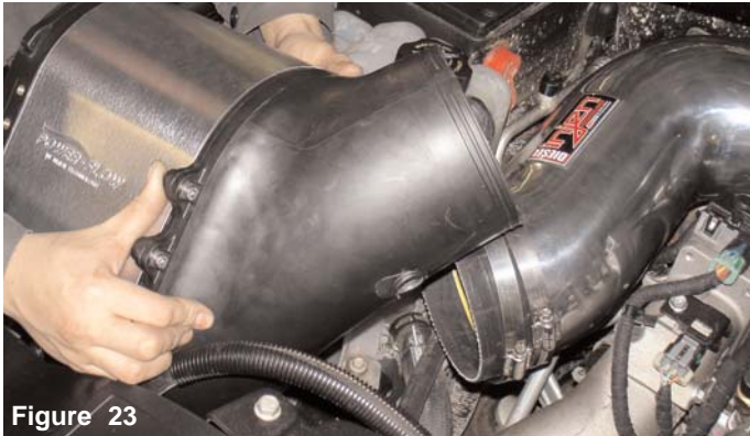
Figure 21 The 5 1/2" straight hose is slipped over the end of the cast intake. Press the straight hose no more than 1" or half the length of the straight hose.
