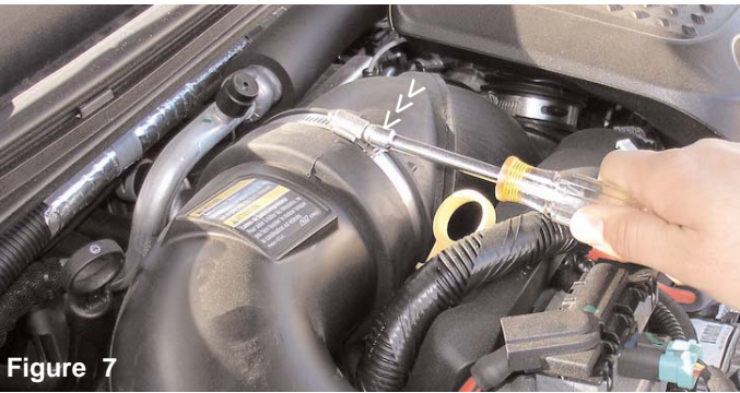
Figure 5 Use the T20 torx bit to loosen and remove the bolts on the mass air flow sensor.
