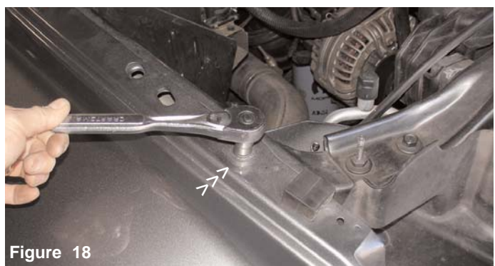
Figure 16 The four m8 x 16mm socket head screws are used to fasten the bracket to the air box cleaner.
