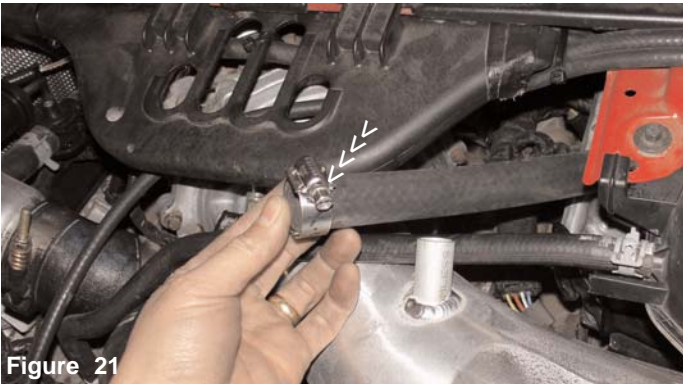
Figure 22 The clamp is now fastened over the 19mm hose as shown above.
