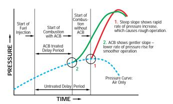
Cylinder pressure measurements made during compression and power strokes illustrate that fuel does not ignite immediately upon injection. Cylinder pressure continues to rise smoothly for a period after injection and rises sharply when combustion starts. The period after fuel injection and before combustion begins is the ignition delay period. By shortening the ignition delay period in high load operations, ACB improves smooth operation.
