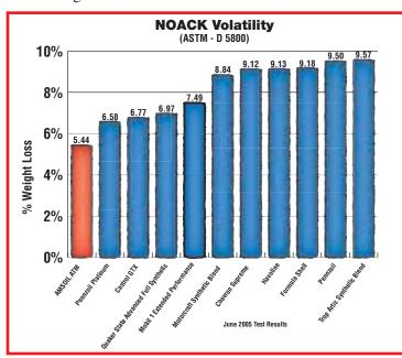
The NOACK Volatility Test determines the evaporation loss of lubricants in high-temperature service. The more motor oils vaporize, the thicker and heavier they become, contributing to poor circulation, reduced fuel economy and increased oil consumption, wear and emissions.
