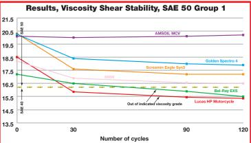
The Viscosity Shear Stability Test determines how well an oil retains its viscosity when submitted to the high-heat and shearing forces within motorcycle engines. Engines operating at high RPMs and those that share a common oil sump with the transmission are particularly subject to high shear rates. The oils that perform well are those that show little or no viscosity change.
