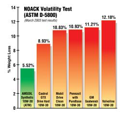
In the Noack Volatility Test (ASTM D-5800), the smaller the evaporative loss, the better an oil functions in heat and that translates into better engine protection plus better fuel economy.
