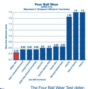
mines the wear protection properties of a lubricant.
