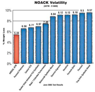
The Noack Volatility Test is a standard test used to measure the evaporation loss of lubricating oils. The low volatility of AMSOIL Synthetic Motor Oil reduces oil consumption, improves fuel efficiency and maximizes engine protection.
