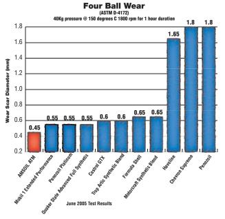
The Four Ball Wear Test determines the wear protection properties of a motor oil by measuring the wear scars created by four metal balls in contact. The smaller the wear scar the better the engine protection.
