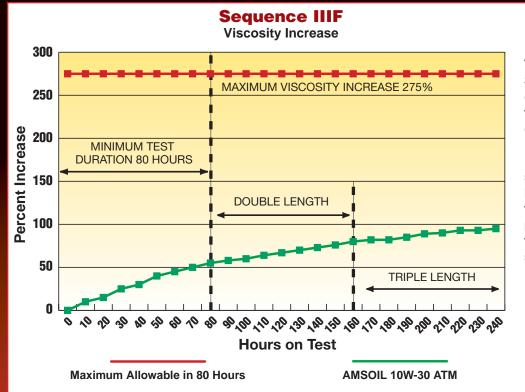
The results of the Sequence IIIF test clearly demonstrate the long-drain capability of AMSOIL 10W-30 Motor Oil. Even after being subjected to a triplelength sequence IIIF test, AMSOIL 10W-30 performed three times better than the standard test limits.
