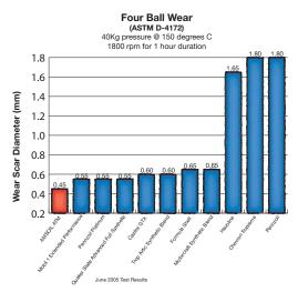
AMSOIL Synthetic Motor Oil provides unsurpassed protection against engine wear. Equipment life is extended, and repairs, downtime and expenses are reduced. The smaller the scar, the better the protection.
