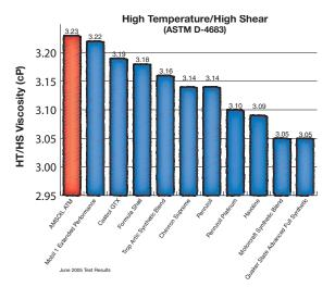
The superior viscosity retention of AMSOIL Synthetic Motor Oil in the face of severe temperature and shear conditions allows it to provide continuous, unsurpassed protection for engine bearings, extending equipment life and preventing wear.
