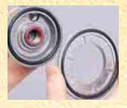
If the kit's gasket is smaller than the original full-flow's, use the adapter plate and adapter plate O-ring with the spin-on adapter.
